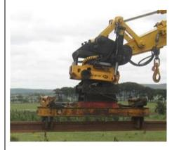
A recent (non-VGC) incident involved a rail beam being used to lift a 60ft section of rail.
