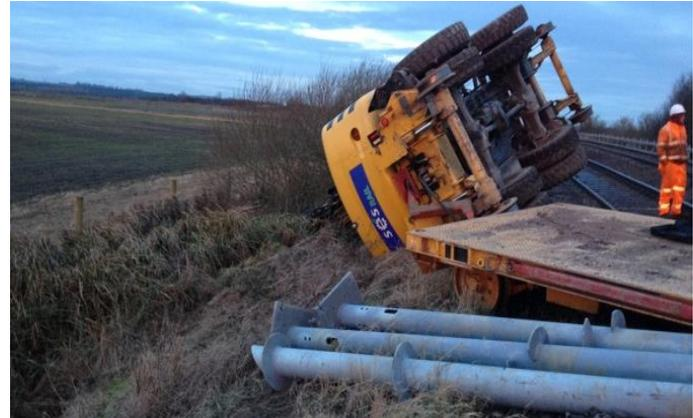
Whilst installing a helical screw pile on the morning of 14 December an Atlas 1604 RRV became unstable, derailed and then overturned. Fortunately no one was injured, however the vehicle remained foul of the line until it could be removed, preventing the affected line being handed back for over 11 hours.
